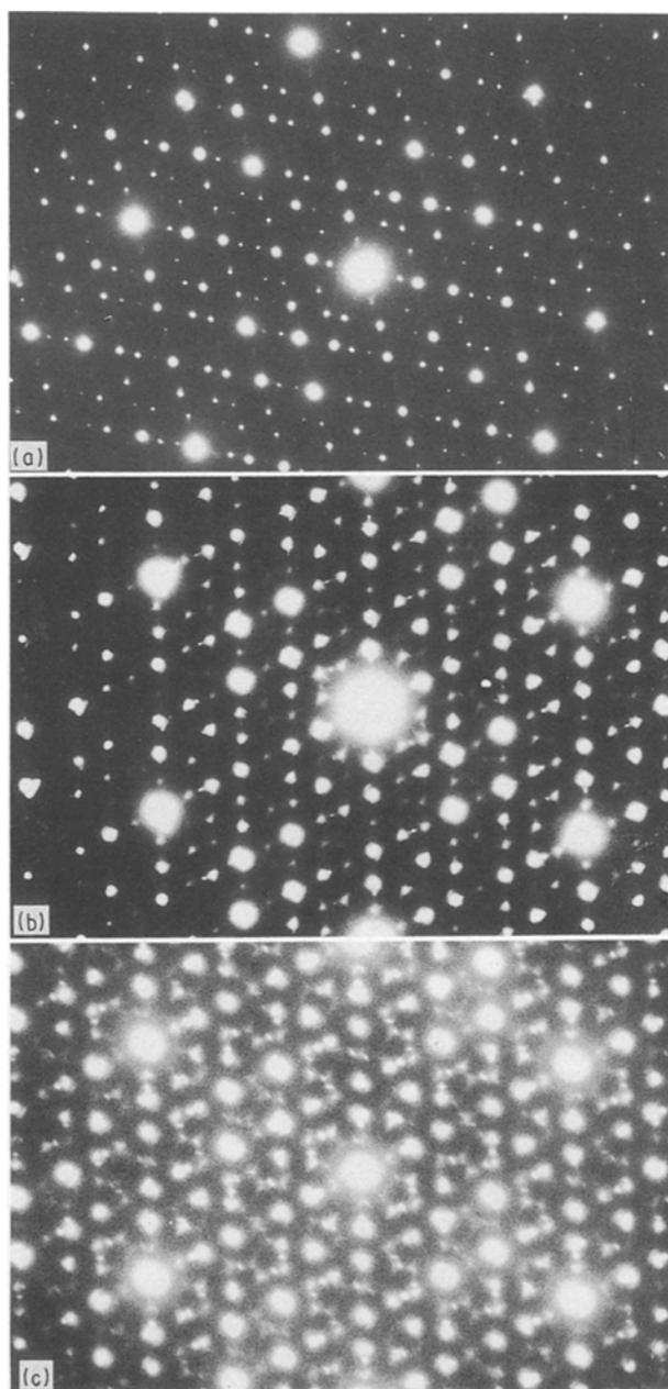
Figure 7 Diffraction patterns from the icosahedral phase along the twofold axis. (a) Before annealing; (b, c) after annealing at 800 °C for 24 h.
