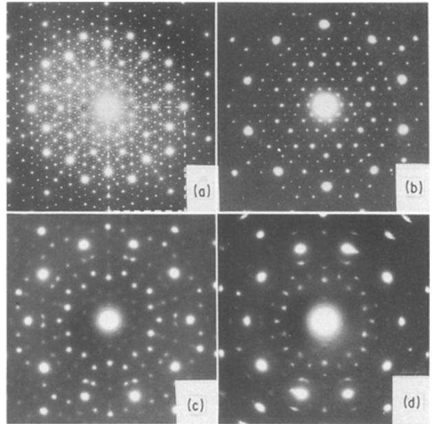
Figure 3 Diffraction patterns from the decagonal phase of Al-Cu-Co-Si along a tenfold axis. (a) Diffraction pattern at the beginning of the experiment; (b, c, d) same diffraction patterns at different electron radiation times. The exposure time is increased from (b) to (d).
