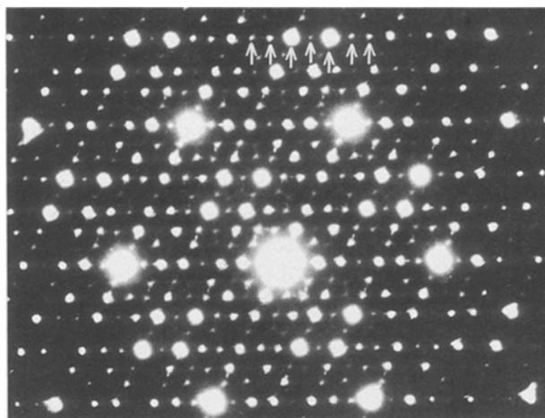
Figure 6 Diffraction pattern from the icosahedral phase along the twofold axis. Periodicity is indicated by the arrows.
