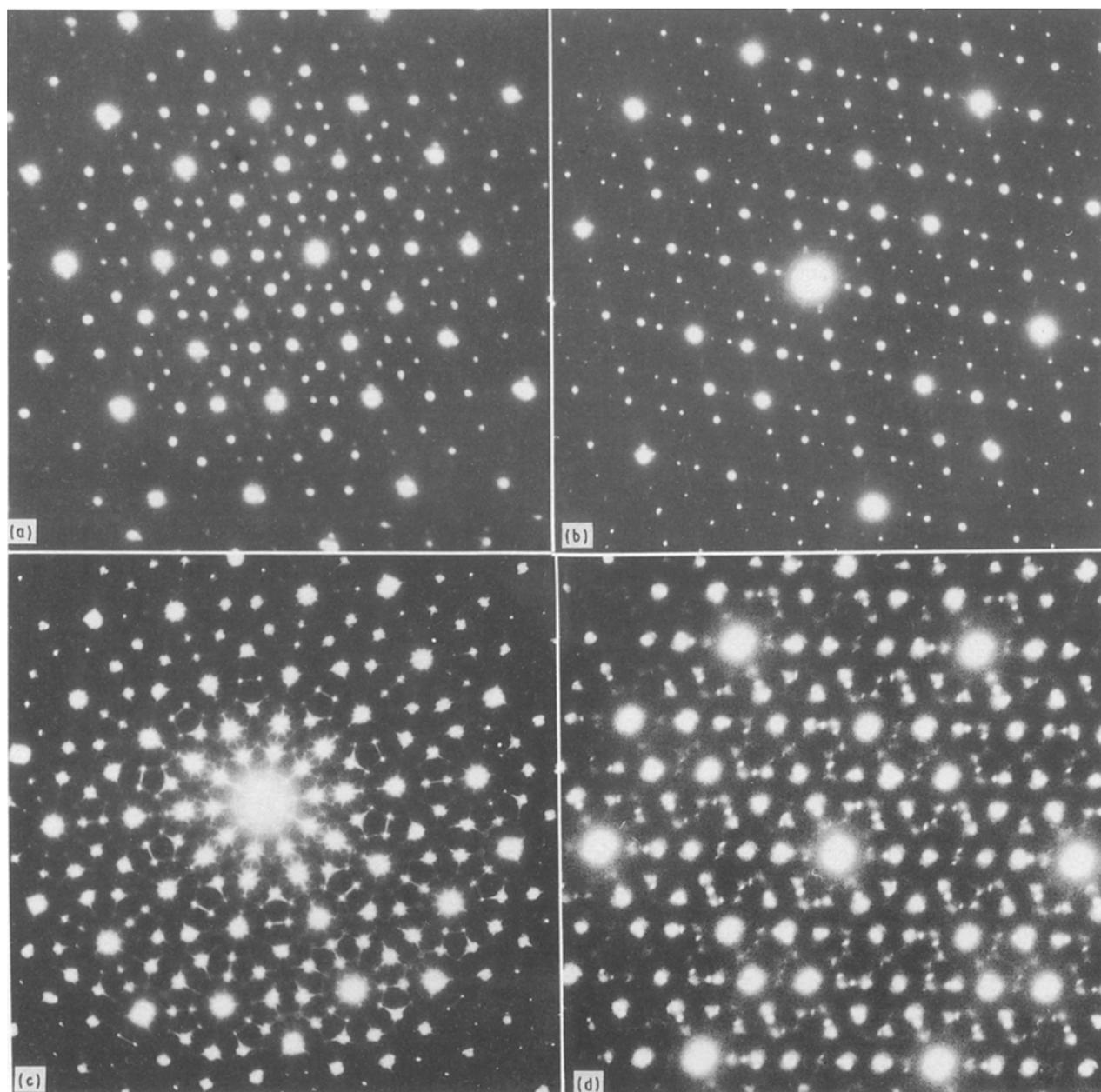
Figure 5 Diffraction patterns from the icosahedral phase of Al-Cu-Co-Fe alloy (a) along the fivefold axis, (b) along the twofold axis, (c) along the fivefold axis after annealing at 800 °C for 24 h, (d) along the twofold axis after annealing.
