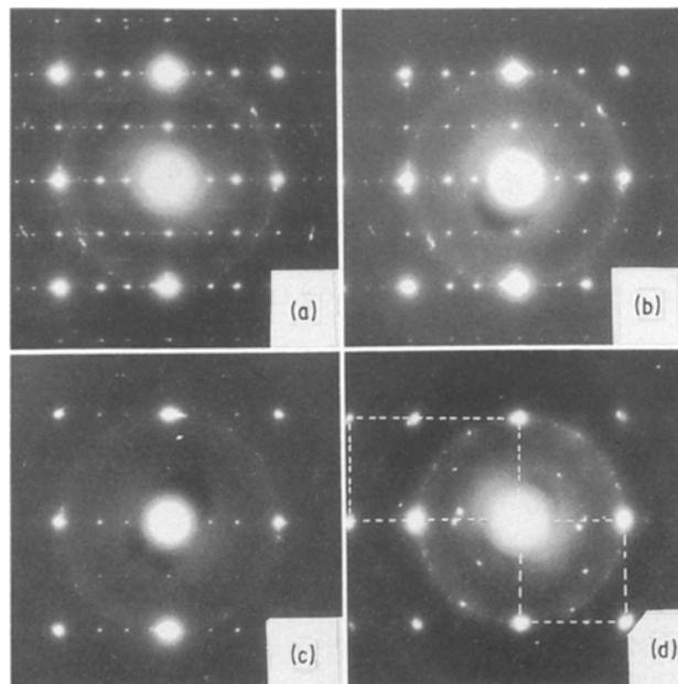
Figure 2 Diffraction patterns from the decagonal phase of Al-Cu-Co-Si along a twofold axis. (a) Diffraction pattern at the beginning of the experiment; (b, c, d) same diffraction patterns at different electron radiation times. The exposure time is increased from (b) to (d).
