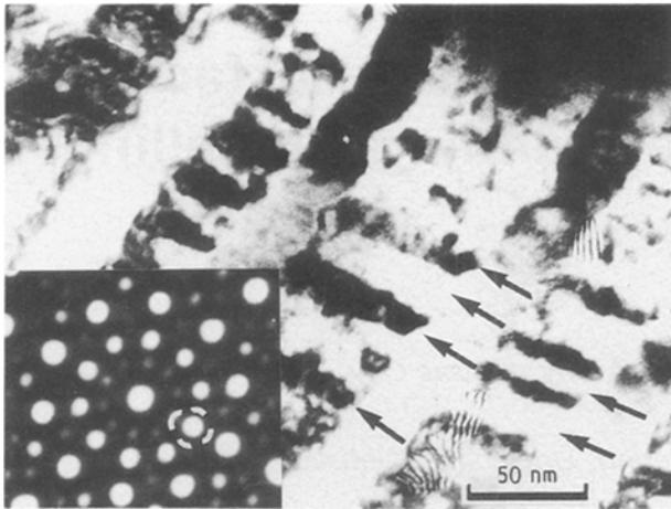
Figure 8 Dark-field image under fivefold diffraction conditions. The dark field is formed with a spot from the second ring of reflections. The contrast features are similar to twinned regions in crystalline specimens.
