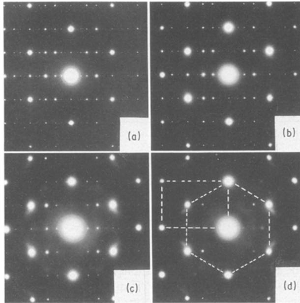
Figure 1 Diffraction patterns from the decagonal phase of Al-Cu-Co-Si along a twofold axis. (a) Diffraction pattern at the beginning of the experiment; (b, c, d) diffraction patterns which correspond to different electron radiation times. The exposure time is increased from (b) to (d).
